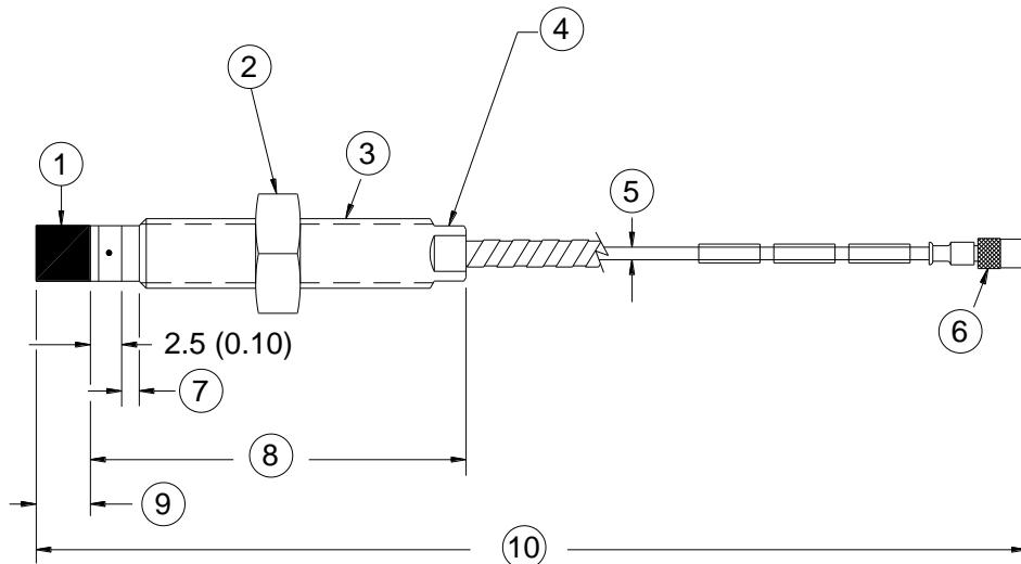
1. Probe tip, 8.0 mm (0.31 in) diameter
