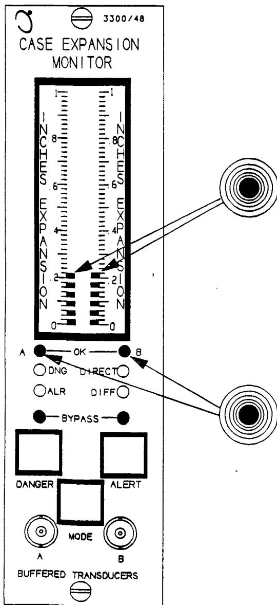
The monitor on this page is giving a signal that a continuing error has been detected during a self test. When a continuing error is detected,
